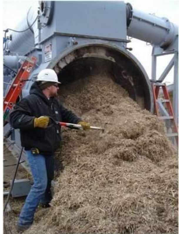
An employee removes feed stock from the ICM gasifier in suburban Wichita, Kan. / Photo supplied by ICM
